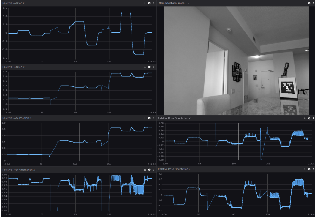
Figure 8: Sample image and pose detection results for hardware AprilTag measurement noise test
