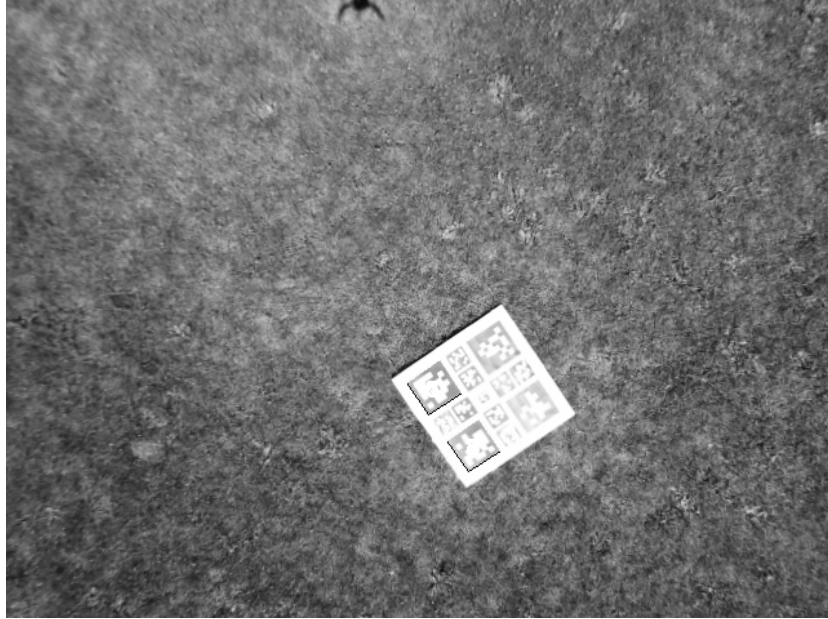
Figure 39: Sample image showing tag image becoming washed out when viewed from above in bright sunlight, leading to only 2 of 13 tags in the bundle being detected
