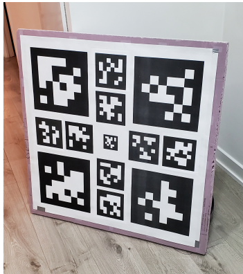
Figure 5: Custom landing target made from nested AprilTags for hardware experiments
