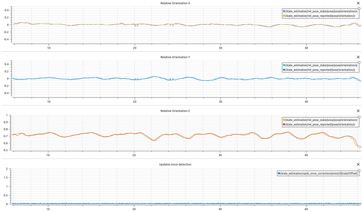
Figure 19: Orientation estimate results for the translation case at a height of 1 m
